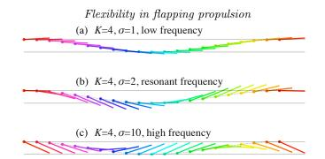
FIGURE 2. Visualizing the emergent kinematics given by Eq. (2.16). A single wing (R = 0, K = 4) is driven at three different frequencies. (a) A low driving frequency produces only slight pitching motions. (b) When driven near resonance, the pitching is much more pronounced. (c) Driving the wing at high frequency results in out-of-phase pitching.
