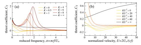
FIGURE 6. Effects of wing inertia. (a) Thrust coefficient versus reduced frequency for the same spring stiffnesses considered earlier, but with a wing/fluid inertia ratio of R = 1. The most compliant wings (yellow curves) can produce negative thrust. (b) Thrust coefficient versus translation velocity for freely swimming wings of different stiffnesses.
