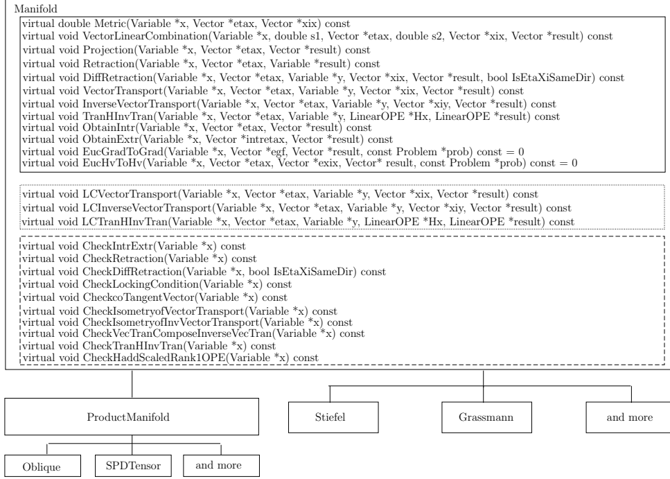
Figure 3: The class hierarchy of manifold-related classes in ROPTLIB. We refer to the documents in the code for the detailed explanations of the functions. {f3}
