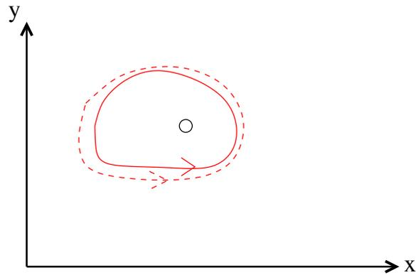
Figure 8: Two limit cycles near a saddle-node of periodics (SNP) bifurcation.
