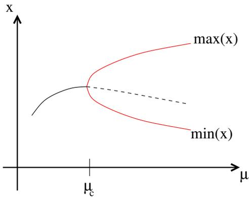
Figure 6: Typical bifurcation diagram near a supercritical Hopf bifurcation. Black=stationary branch, Red=min and max of stable periodic branch.
