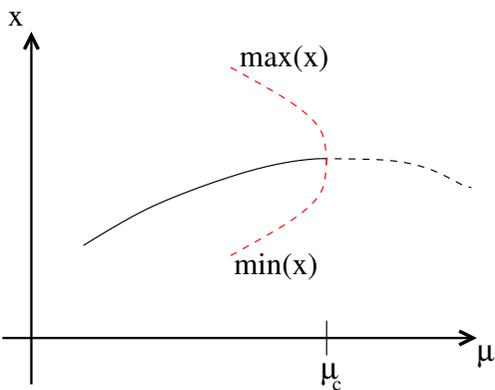
Figure 7: Typical bifurcation diagram near a subcritical Hopf bifurcation. Black=stationary branch, Red=min and max of unstable periodic branch.
