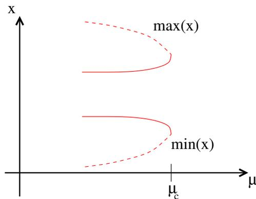
Figure 9: At an (SNP) bifurcation two periodic branches, one stable and the other unstable, join together at a turning point. In the diagram there appears to be two turning points, but there is only one since the upper curve represents the maximum of the limit cycles and the lower curve represents the minimum.
