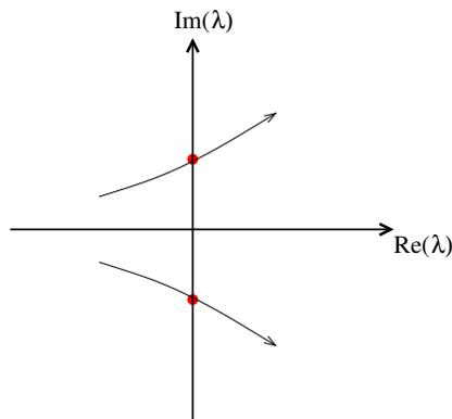
Figure 4: The eigenvalues cross through the imaginary axis at a Hopf bifurcation. The red points indicate the Hopf bifurcation.
