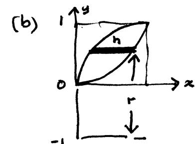
$$t = \frac{y}{h}, \quad h = \sqrt{y} - y^2, \quad \delta V = 2\pi r h \delta t + o(\delta t) \\ r = 1 + y \quad = 2\pi(1+y)(y^{1/2} - y^2) \delta y + o(\delta y)$$
