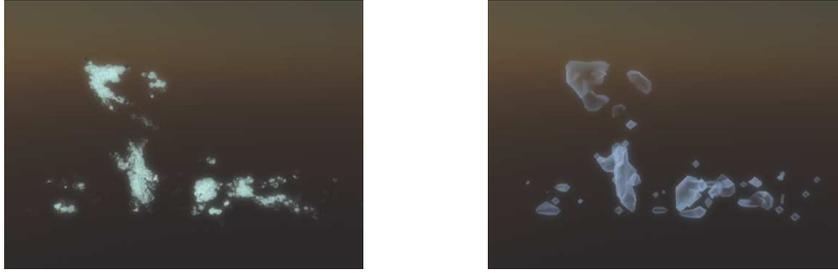
**Figure 4:** Left: droplet positions. Right: a level set of the extrapolated density field shows good agreement with droplet position. See section 2.2.2 and the Appendix for more details.
