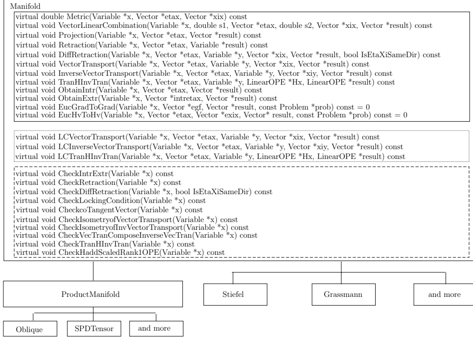
Figure 3: The class hierarchy of manifold-related classes in ROPTLIB. We refer to the documents in the code for the detailed explanations of the functions.
