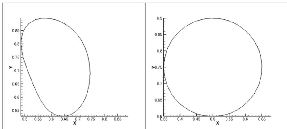
**Figure:** single vortex problem ( $T = 1/2$ )  $64 \times 64$  midway through the simulation and at the end. Shape deforms back to a circle. Two materials. At  $t = T = 1/2$ , symmetric difference error is  $7.4E - 5$  (operator split symmetric difference error:  $14.3E - 5$ )
