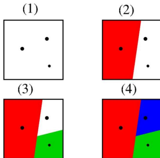
Slope of Red (solid) cut determined first, then slope of green (fluid 1) cut determined second. Blue material occupies remaining unfilled region.
