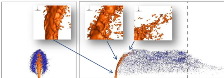
Figure 6. Front (a) and side view (b) of the jet at  $t = 1.686$  ms. The jet calculated by CLSVOF on the Eulerian grid is represented by the rendering of the 0 level set iso-surface. The spray (Lagrangian) is shown as a scatter of spheres whose diameter is scaled to the plot. The continuous lines delimit the boundary domain, the dashed line is the trace of the sampling plane. Different segments of the iso-surface only, from near injection to breakup, are also displayed in the three inserts.
