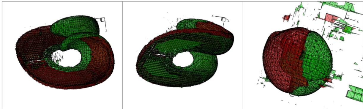
**Figure:** single vortex problem ( $T = 3$ )  $64 \times 64 \times 64$  midway through the simulation and at the end. Shape deforms back to a sphere. Three materials. Initially, Material 1 (red) is the left half of the sphere, and Material 2 (green) is the right half. At  $t = T = 3$ , symmetric difference error is 0.00158 for material 1, 0.00104 for material 2, and 0.00188 for material 3.
