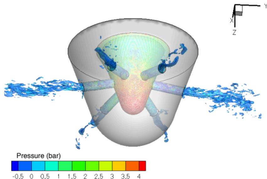
**Figure:** Snapshot of a simulation of liquid injection in a Bosch six-hole vertical diesel nozzle. Effective fine grid resolution 640x640x256.
