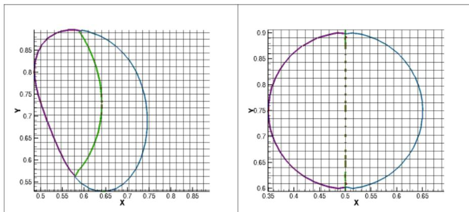
**Figure:** single vortex problem ( $T = 1/2$ )  $64 \times 64$  midway through the simulation and at the end. Shape deforms back to a circle. Three materials. Initially, Material 1 (red) is the left half of the circle, Material 2 (green) is the right half, and Material 3 (blue) is the space outside the circle. At  $t = T = 1/2$ , symmetric difference error is  $9.6E - 5$  for material 1,  $10.1E - 5$  for material 2, and  $14.8E - 5$  for material 3.
