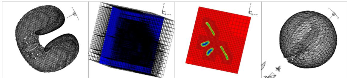
**Figure:** 3D single vortex problem ( $T = 3$ )  $64 \times 64 \times 64$  midway through the simulation and at the end. Shape deforms back to a sphere. Two materials. At  $t = T = 3$ , symmetric difference error is 0.00189 (operator split symmetric difference error: 0.00202)
