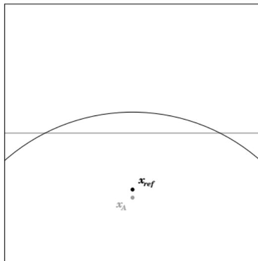
**Figure:** The reference centroid,  $x_{ref}$ , does not coincide with the exact centroid,  $x_A$ , for a parabolic interface cutting the cell. The difference between the two centroids is proportional to the curvature.
