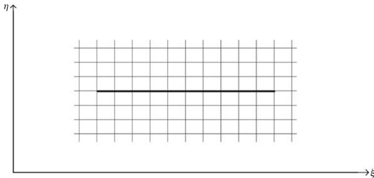
FIGURE 10. Mapping of the aerofoil into a slit in the  $w$  plane.
