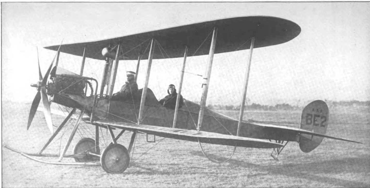
R.A.F. TYPE B.E.2. As flown at the International Competition in August, 1912. The forerunner of the later B.E.2 Types. Speed: Max. 70 m/h.; not inherently stable.
