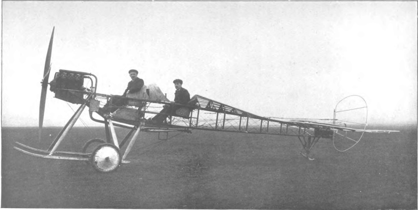
SKELETON OF TYPE B.E.2. Showing position of Tank, Seats, Engine, and Body structure. Illustrates the extent of the vulnerable target presented by an Aeroplane.
