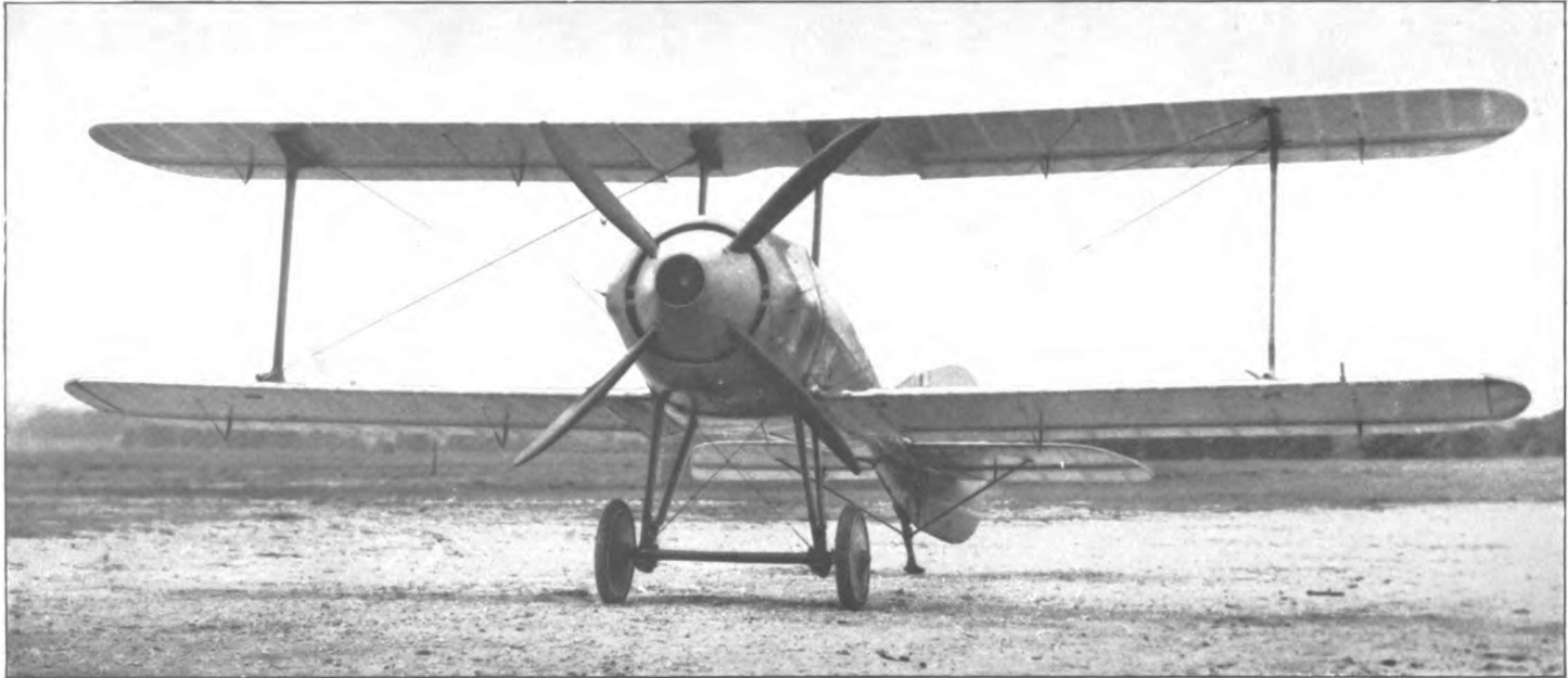
R.A.F. TYPE S.E.4. Single Seat Reconnaissance Machine. Maximum Speed over 130 Miles per hour.
