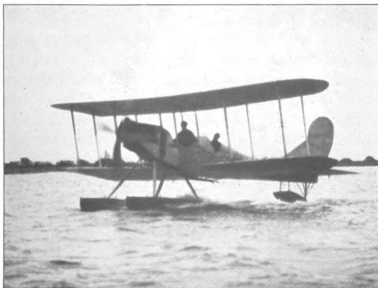
HYDRO-AEROPLANE H.R.E.3. R.A.F. Design for the "Naval Wing" (Now R.N. Air Service) in 1912.
