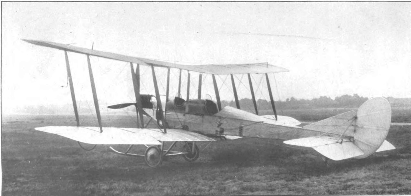
EARLY (EXPERIMENTAL) MODEL OF B.E.2c Calculated and Demonstrated as inherently stable by the late Mr. E. T. Busk. Compare Plate III.
