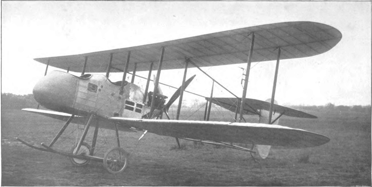
R.A.F. TYPE F.E.2. Designed to carry gun weight 300 lbs. Wings interchangeable with B.E.2. Speed: Max. 69 m/h. Climb 1,000 ft. in 3½ minutes. Designed and built in 1913.
