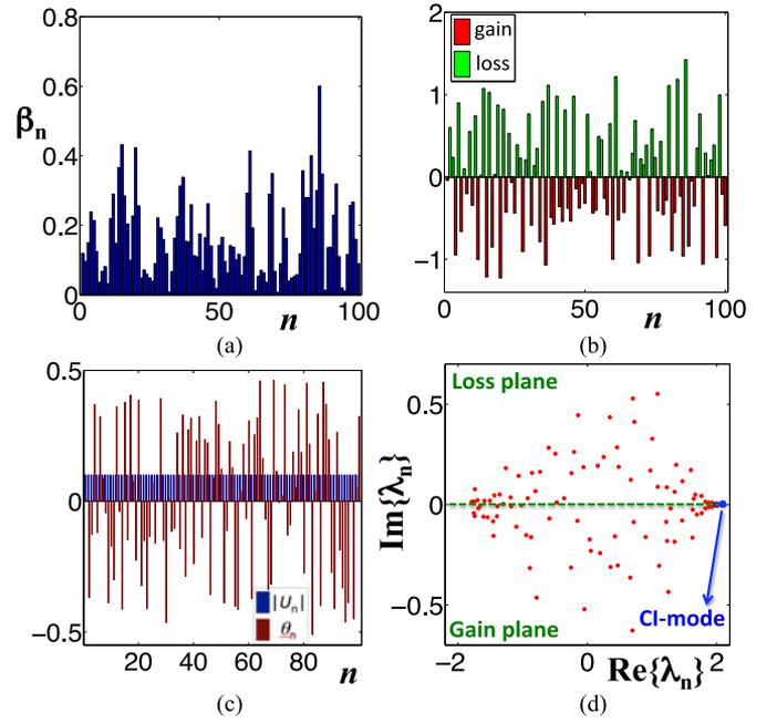
Fig. 4. CI-mode (with  $\lambda = 2$ ,  $g = 1$ ) in a disordered lattice of  $N = 100$  waveguides with a random phase. In particular, (a) real part and imaginary parts of the refractive index per waveguide, (b) gain and loss per channel, (c) the amplitude and phase of the CI-supermode, and (d) eigenvalue spectrum in the complex plane. The eigenvalue of the CI-supermode is denoted with a blue circle.
