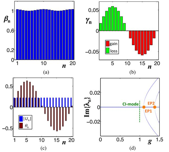
Fig. 2. CI-mode (with  $\lambda = 3$ ) in a lattice of  $N = 20$  waveguides for a periodic phase. In particular, (a) real part of the refractive index per waveguide, (b) gain-loss distribution per channel, (c) the amplitude and phase of the CI-supermode, and (d) the imaginary part of all eigenvalues versus  $g$ . The exceptional points (EP) are denoted with orange dots and the value of  $g$  for which the CI-mode exists with a dashed green line in (d).
