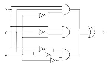
(e) Sketch the logical network that has the same output as F, and uses the order of operations given in the expression in part (b).
