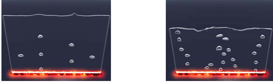
Figure 3: Circulation increase in a boiling flow: (a) early "straight" pattern (b) late development mixing pattern
