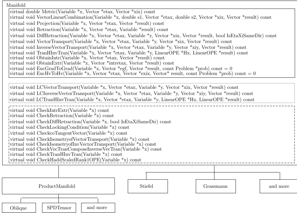
Figure 3: The class hierarchy of manifold-related classes in ROPTLIB. We refer to the documentations in the code for the detailed explanations of the functions.
