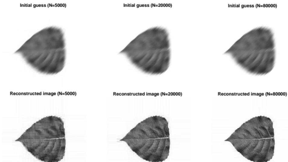
**Figure:** Initial guess by running power method for 50 iterations and the reconstructed image for  $N = 5000, 20000, \text{ and } 80000$ . Computational time: 2-3 mins.
