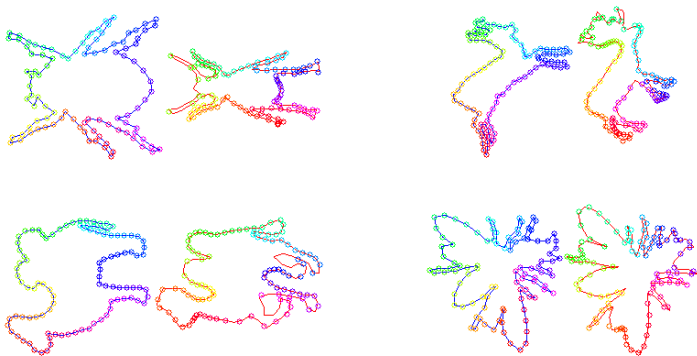
Figure: Applying best rotation and reparameterization to one of the curves. The colors indicate corresponding points on the two curves.
